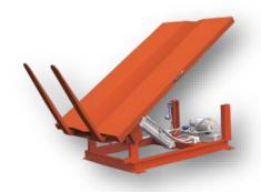
**Ecoa Hue series** heavy-duty electrohydraulic tables offer capacities of 2,000 to 10,000 lbs., tilt angles to 90 degrees and a wide range of platform sizes. Feature a lowered height of 10-12". Includes a limit switch and mechanical stops in both directions.
