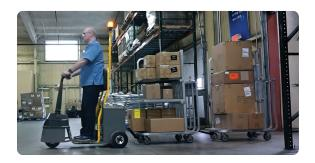
"Our custom trailers were developed for the Dex to feed our production lines more efficiently while reducing worker fatigue and improving their safety."
