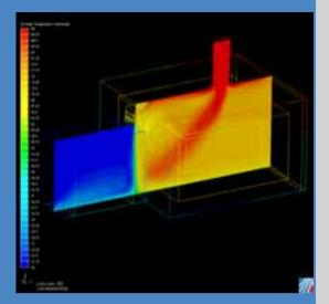
The above Computational Fluid Dynamics (CFD) snapshot demonstates how air curtains provide separation at an open door, keeping valuable heated air inside.
