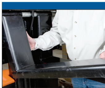
Adjustable fork carriage allows forks to be repositioned to best accommodate loads (straddle only).
